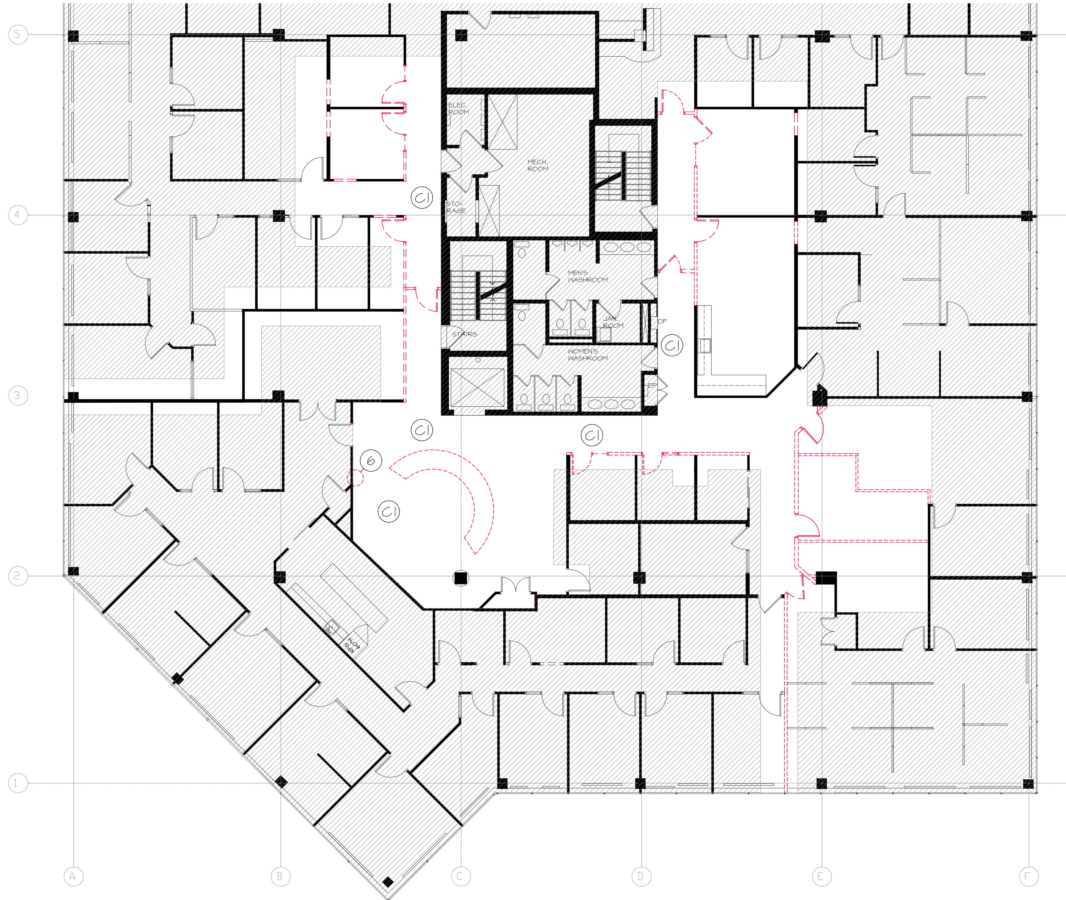
1 ID-1.1 DEMOLITION PLAN SCALE: 1/8"=1'-0"
